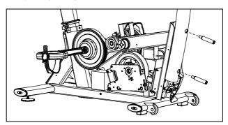
Figure 6: Bolting the upright support into place
